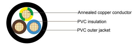
Conductor: Annealed copper conductor to AS/NZS 1125
