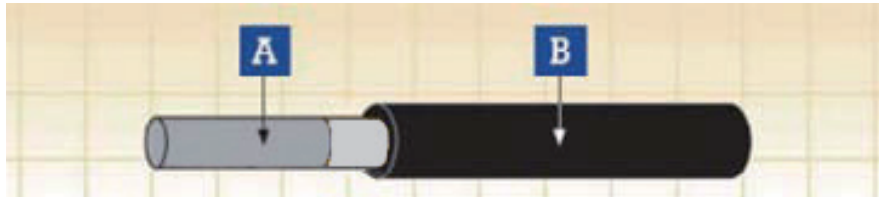
A. Conductor B. Insulation
